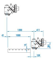
**DIRECT SPINDLE HEAD 4.000 rpm (HFK-225)**
